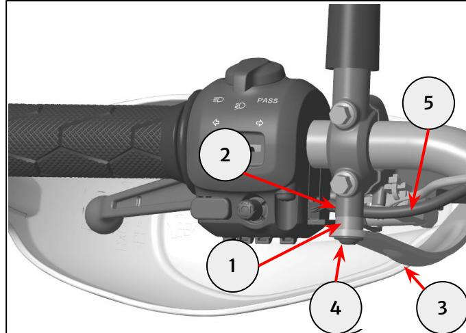
**4** Locate the bracket (1) on the front master cylinder clamp mount boss (2). Fit the M6 x 12mm fixing (3). Align the bracket (3) to locate the fixing in the forward position of the bracket slot.
