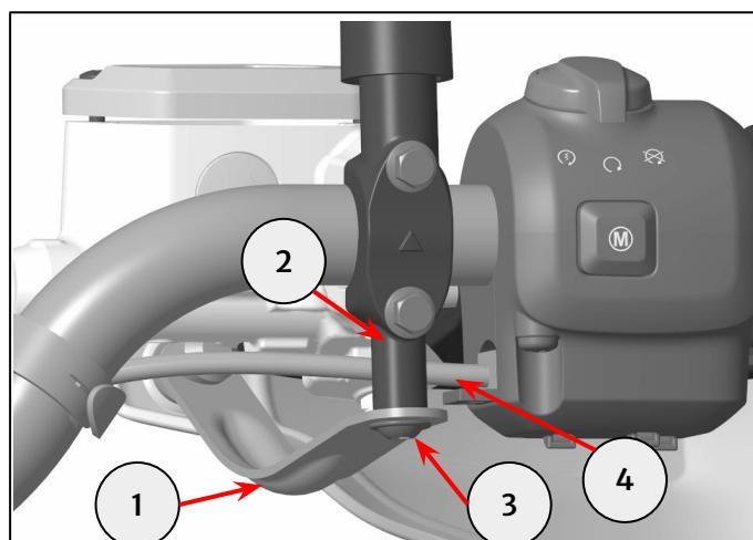
**5** Fit a bar end spacer (1), handguard (2) and reused bar end weight (3) to the handlebar end, as shown.
